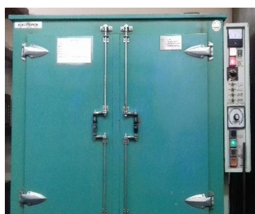
Figure 3 Hot air oven
